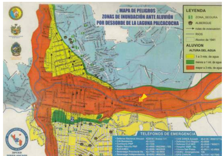
Highlighted in orange, the hazard map shows those city areas of Huaraz which are particularly threatened by high waters and a flood from the glacial lake Palcacocha (the arrow in the town center marks the location of the home of the Luciano Lliuya family).
